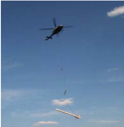
A helicopter is seen here with suspended geophysical instruments.
