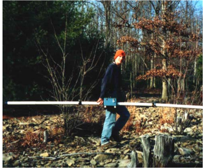
Neil Wolfe, a Lock Haven University geology student, uses an EM31 instrument to measure conductivity in the Huling Branch area.
